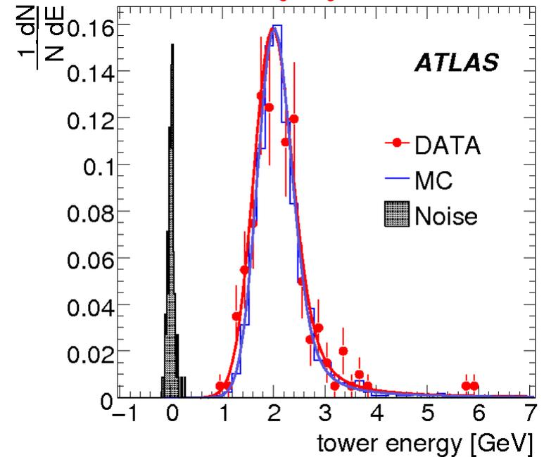
Example of the total muon response passing through the calorimeter at  $|\eta|=0.35$
