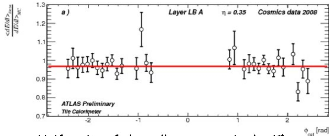
Uniformity of the cell responses in the 1<sup>st</sup> radial sampling, as a function of azimuth  $\phi$ , no/little statistics for horizontal muons
