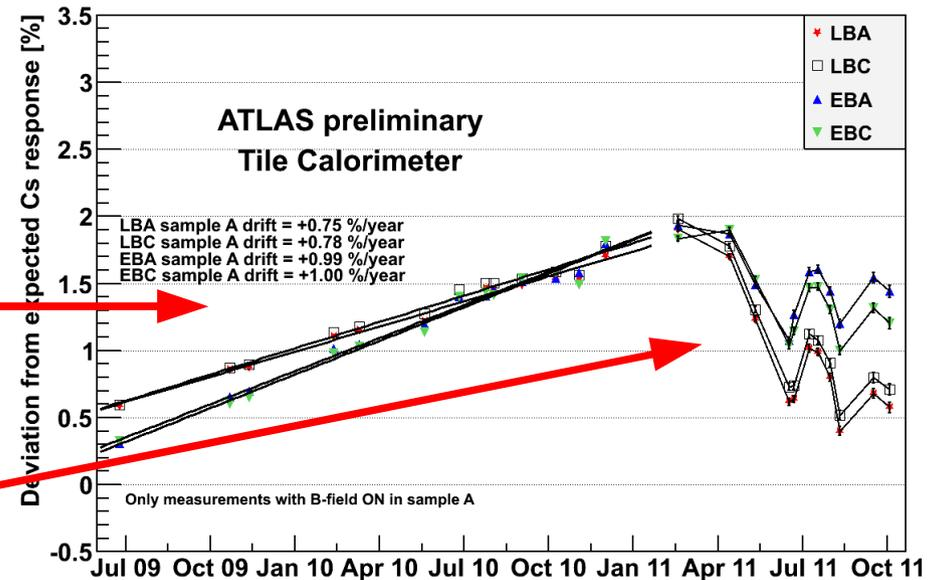
We monitor the gain changes and apply appropriate corrections to Cs calibration constants in order to keep the calorimeter response stable within 0.5%
