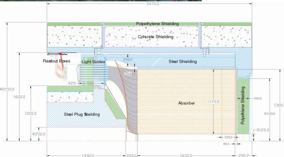
Detailed description of HF calorimeter can be found at – EPJ, C53, N 1 (2008)
