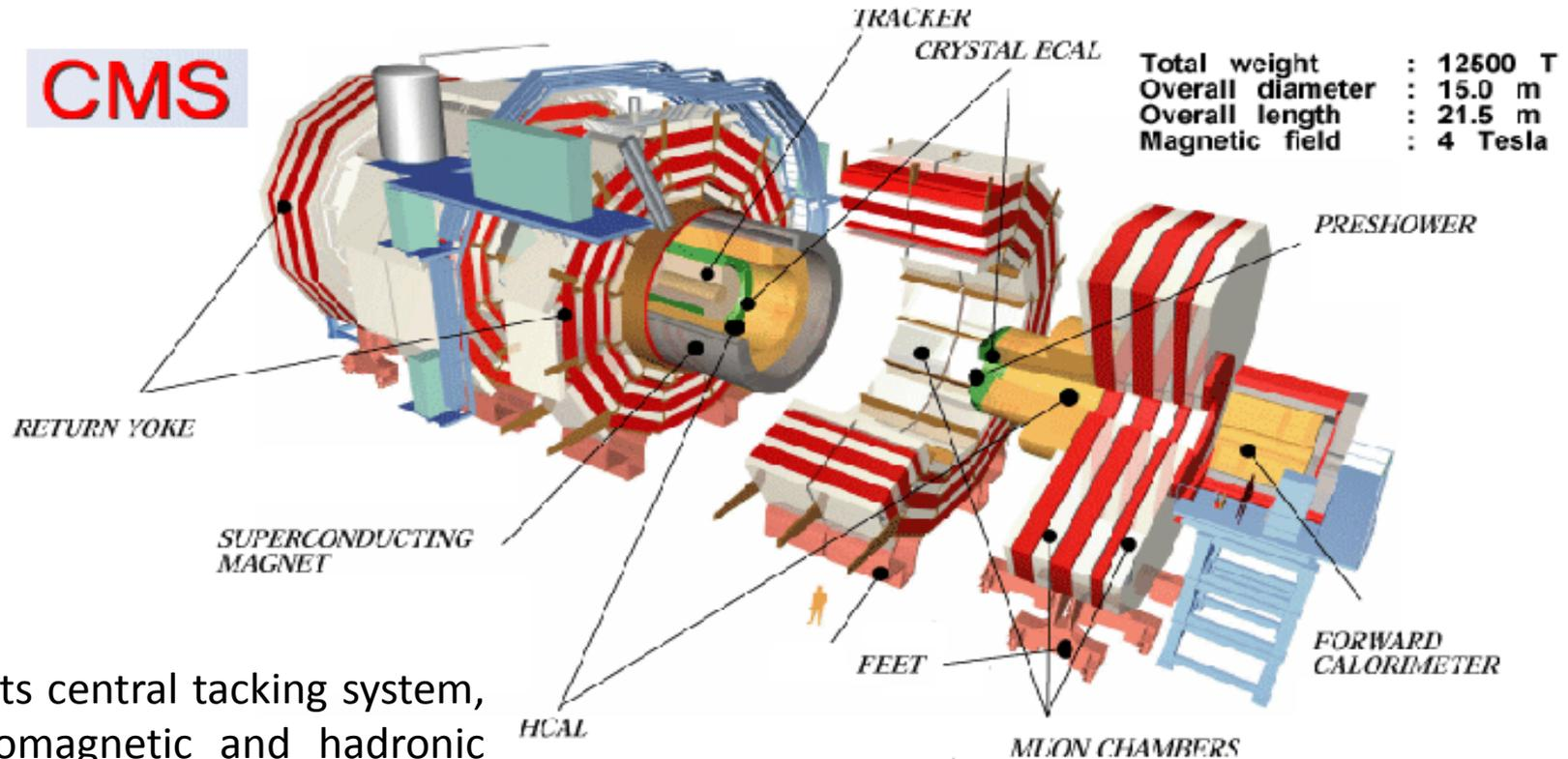
consists central tracking system, electromagnetic and hadronic calorimeters, superconducting magnet providing 4 Tesla magnetic field and muon system.
