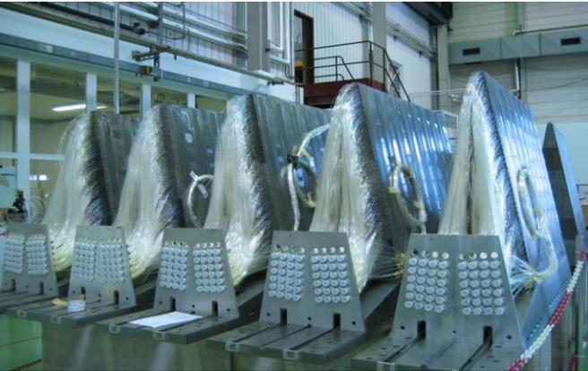
Two compartments ElectroMagnetic and HADronic defined by the embedded fiber length
