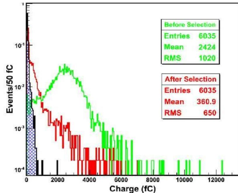
Reduction of the unwanted window events after selecting those signals with high correlation between the channels (right-red distribution). Window events will produce signals in some of the channels but not all of them (uncorrelated) as seen in the event distribution before the selection (green).
