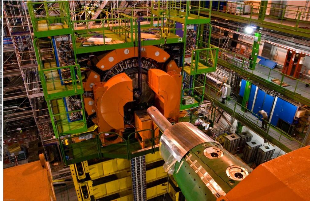
HF calorimeter is composed with two identical parts located at the + and – ends of the CMS detector
