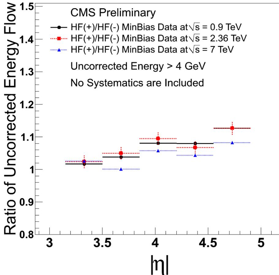
In the figure the ratio of energy flow from HF(+) to energy flow from HF(-) is shown. Uncorrected energy measurements are used and systematic uncertainties are under study
