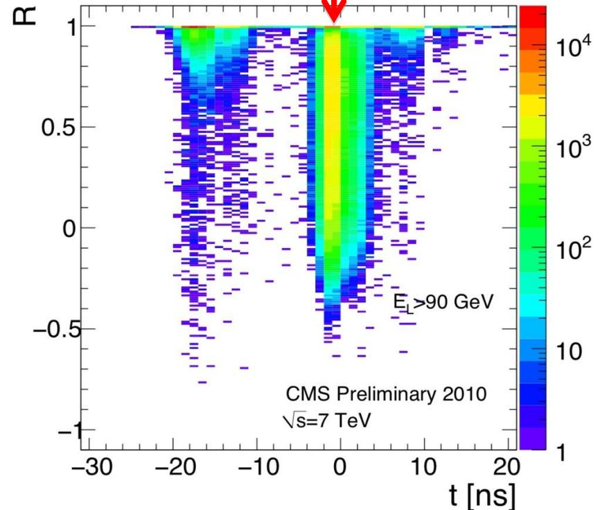
R ratio versus reconstructed time for short (left) and long (right) fiber hits having  $E > 90$  GeV in 7 TeV collision data ( $\sim 1 \text{ nb}^{-1}$  minimum bias data).
