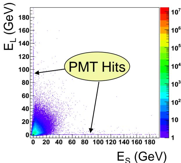
R is used to identify PMT hits in the short fibers. For long fibers an isolation criterion is used to avoid misidentifying EM showers as PMT hits
