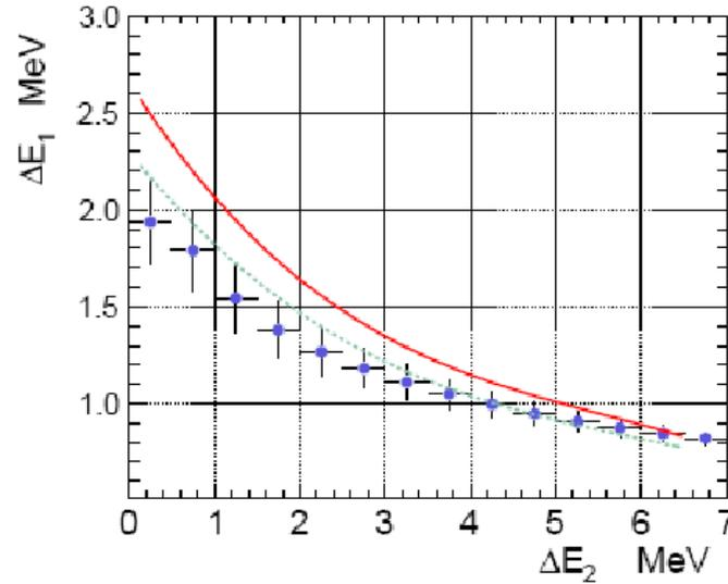
Total energy deposit and reconstructed kinetic energy correlation for stopped deuterons and stopped in the 3<sup>rd</sup> layer protons
